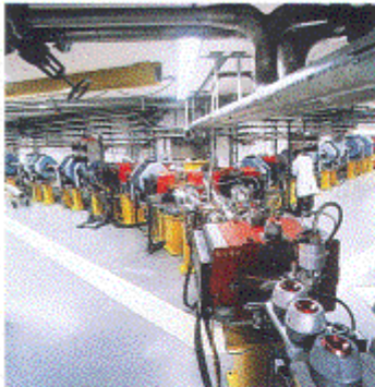
Particles pass from the Linear Injector for LEP, LIL, into the Electron Positron Accumulator at this junction.
