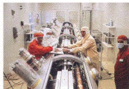
Engineers at work on one of LEP2's superconducting accelerating cavities.
